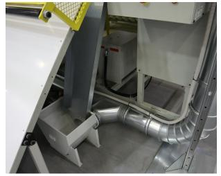
The Waste-exit clean factory system eliminates inefficient handling of scrap waste by automatically collecting, transporting, and depositing waste into an optimally positioned bin or baler. Automatically moving scrap increases work-cell efficiencies 10-30 percent and eliminates unnecessary labor. Waste-exit also removes 91 percent of airborne grit that destroys sewing equipment and computers.
