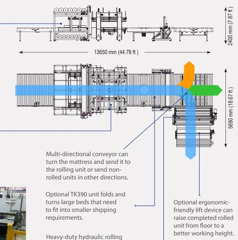
device is capable of rolling up to three units per minute. The unique, adjustable diameter features allow various-sized products to be wrapped at optimum diameter sizes – from 25-45 cm diameter (or 30-55 cm
