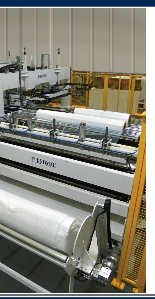
TK381 is a flexible system that can be combined with various material-handling components to fit your space and automation needs. The TK381/1 can wrap units 25-45 cm in diameter while the TK381/2 can wrap units 30-55 cm in diameter.
