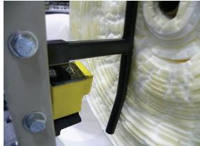
Based on customer feedback, features such as optional, wireless low-material sensors have been added to increase productive runtime.
