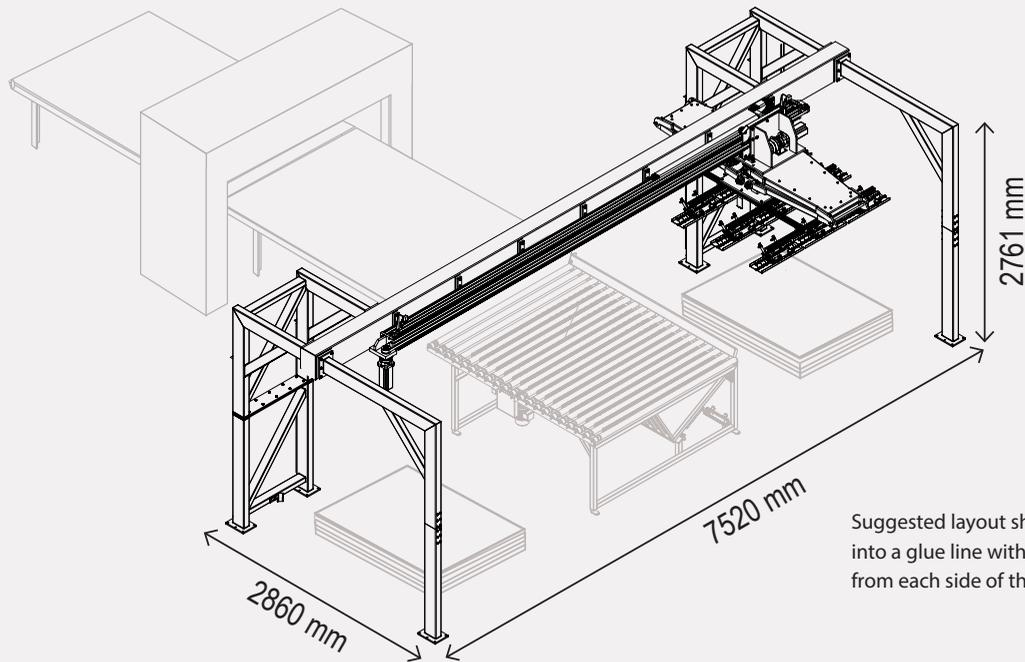
Suggested layout shown here feeds foam layers into a glue line with stacks of foam being loaded from each side of the infeed conveyor.
