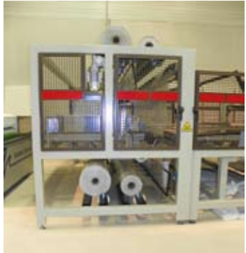
ME105 has capacity to hold 5 rolls of film.
