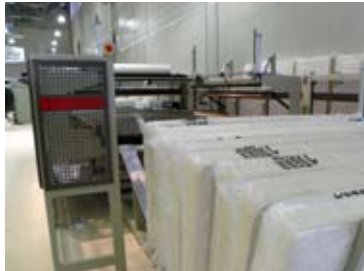
Optional cart stacker automatically loads finished units onto awaiting cart.
