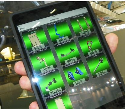
The Portable HMI handheld quilter operations tablet puts machine operations at your fingertips and can reduce downtime with powerful, mobile maintenance tools. It comes with a magnetic charging cradle that mounts to the guilter control cabinet for convenient wireless charging of the device.
