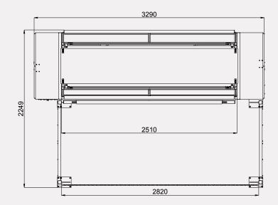
The GS15 flat goods cutter trims non-woven materials to size. It has a built-in panel catcher and programmable operator panel for loading product specifications. The GS15 can trim, cut, and fold six panels per minute and is accurate to within (+/-) 3 mm.
