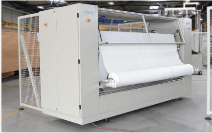
\* Standard machine is equipped to use a single roll of goods. Optional roll holders are available for up to 3 rolls.
