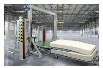
The PS90 automated system transfers various forms of spring units, finished mattresses, and other units to carts or other transport equipment. Its use of motorized belt conveyors eliminates the risk of damage to the units that may be caused by mechanical-picking devices.
